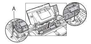
10 Push the toner cartridge to make sure it is properly set in the machine.
